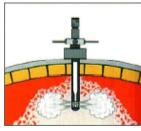
Cardox consists of a high strength reusable steel tube filled with a liquid carbon dioxide, a chemical heater and a rupture disc. When energised by the application of a small electrical charge, the chemical heater instantly converts the liquid carbon dioxide to a gas. This conversation expands the CO2 volume and builds up pressure inside the tube to burst. This releases the CO2 - now 600 times the original volume through a special discharge nozzle to create a powerful
